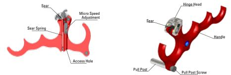
**TIP:** The adjustment on the Micro III is very fine and hard to see. Place your finger on top of the sear while turning the screw. This will allow you to feel the sear move while you make very fine adjustments for speed.
