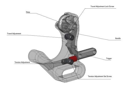
**NOTICE:** The Eagle is a single sear release, so it is possible to set it too light to engage. Test the release for engagement before you pull your bow with it. Turn the screw counter clockwise to increase the sear engagement. The trigger pressure is independently adjustable. Loosen the trigger pressure set screw and rotate the trigger pressure clockwise to increase the tension. Rotate the screw counter clockwise to decrease the tension.
