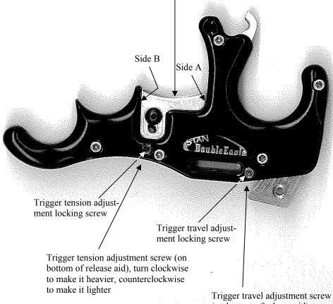
Trigger travel adjustment screw (on bottom of release aid), turn clockwise to reduce travel, turn counter clockwise to increase travel
