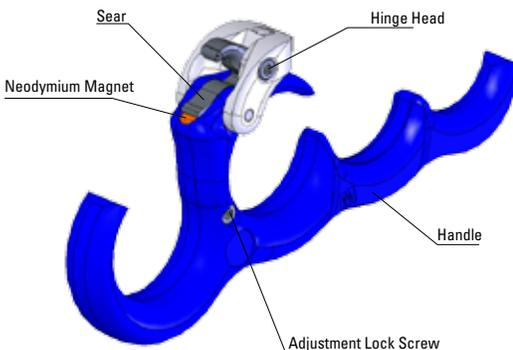
**Warning:** Never allow Neodymium magnets near a person with a pacemaker or similar medical device. The strong magnetic fields of the magnet can affect the operation of such devices. Neodymium magnets will lose their magnetic properties if heated above 175° F (80°C.)
