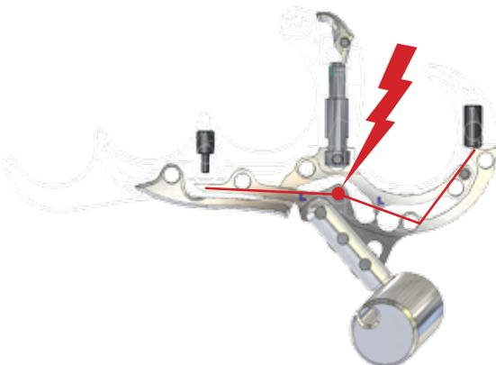
**Caution** - When making your initial adjustments, be careful and do not tighten both the tension adjustment and travel adjustment down together. Doing so will bend the trigger over its center point. When you feel an adjustment get firm or tight while turning, STOP!
