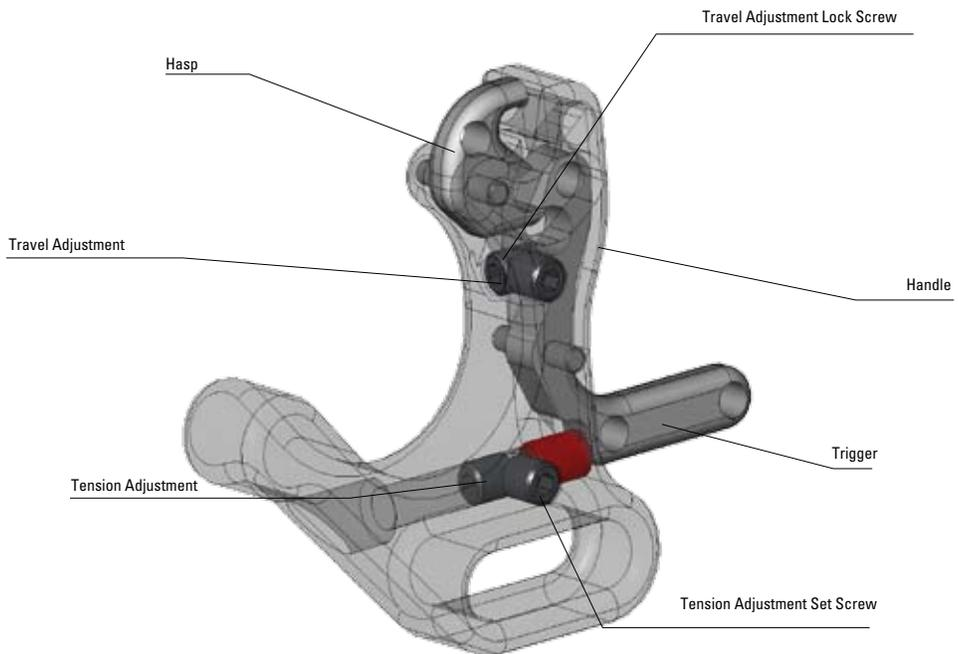
**NOTICE:** The Eagle is a single sear release, so it is possible to set it too light to engage. Test the release for engagement before you pull your bow with it. Turn the screw counter clockwise to increase the sear engagement.
