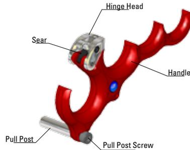
**TIP:** The adjustment on the Micro III is very fine and hard to see. Place your finger on top of the sear while turning the screw. This will allow you to feel the sear move while you make very fine adjustments for speed.
